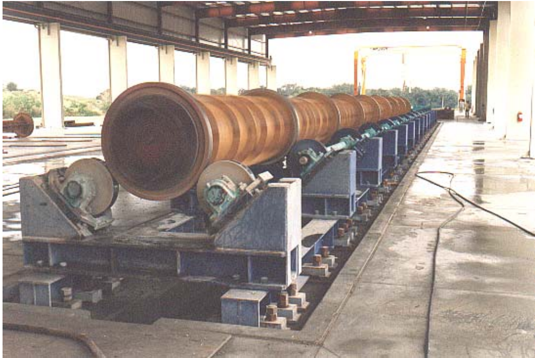
Fig. 8 The centrifuge process for an antenna mast (Photo: Pfeleiderer)
